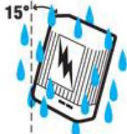
Protected against vertically falling drops of water with enclosure tilted up to 15 degrees from the vertical.
